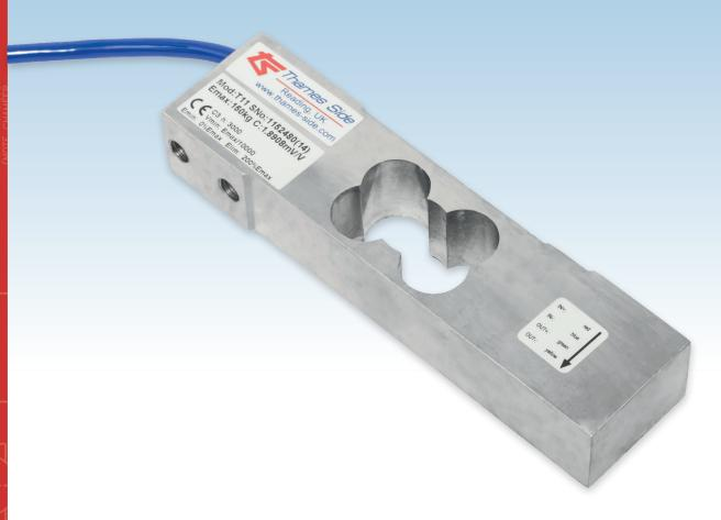
This double bending beam single point load cell is manufactured from high quality alloy steel and nickel plated. Its design allows for high accuracy weigh measurement with off-centre loads and it's potted and sealed to IP66.
