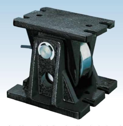
The T95 range comprises of a stainless steel load cell complete with tough, painted mounting assembly. Although the assembly is used in compression, the cell is mounted in a pendulum and operated in tension. This ensures that the load point is always maintained through the central axis of the cell, even when the assembly is subjected to considerable movement or misalignment.
