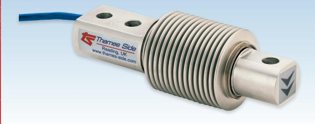
This fully welded stainless steel bending beam load cell is hermetically sealed to IP68 / IP69K and can be used in the harshest industrial environments. It is suitable for weighing platforms, bag fillers, belt weighers and tank weighing in the Food Processing, Chemical, Pharmaceutical and general Bulk Handling industries.
