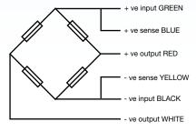
The 2 sense wires are especially important with long cables and wide temperature ranges.
