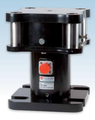
A stainless steel compression load cell housed in an integral mounting assembly, which is ideal for general commercial weighing of large tanks, silos and vessels, particularly in the cement, minerals and coal industries. The design ensures optimum performance and eliminates many traditional problems encountered during the installation of high capacity weighing systems. The T30 load cell and mounting assembly are supplied as a complete locked unit, ready to install.
