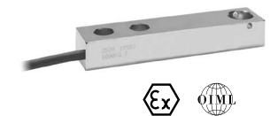
It has high immunity to shock or side loading, and is available in 2 mV/V sensitivity and is approved to OIML 6000 divisions.
